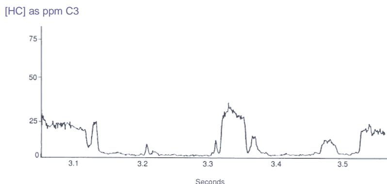
The HFR400 is also used in field studies. This graph shows the response to continuous atmospheric release of propane at a range of 100m, height 2m with a wind speed of 7m/s.
