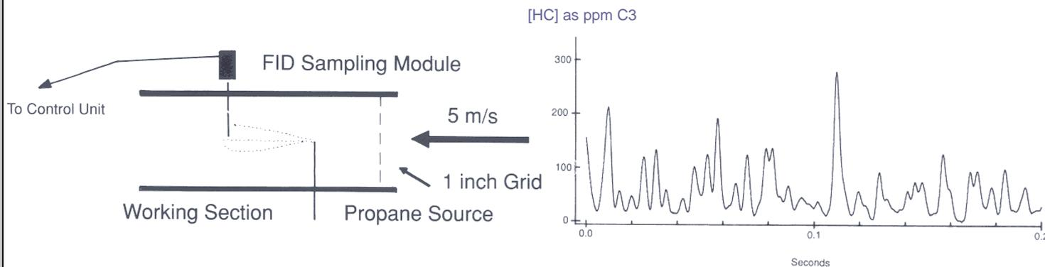
The schematic diagram shows a wind tunnel fitted with a 1 inch grid. Propane is released from a point source upstream and an HFR400 sampling module monitors concentration fluctuations at a station downstream. The graph shows typical concentration fluctuations resulting from such an experiment.
