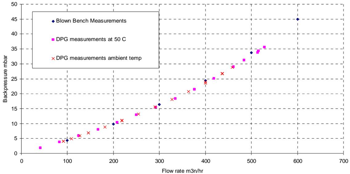
**Figure 1 Pressure drop vs flow rate for DPF**
