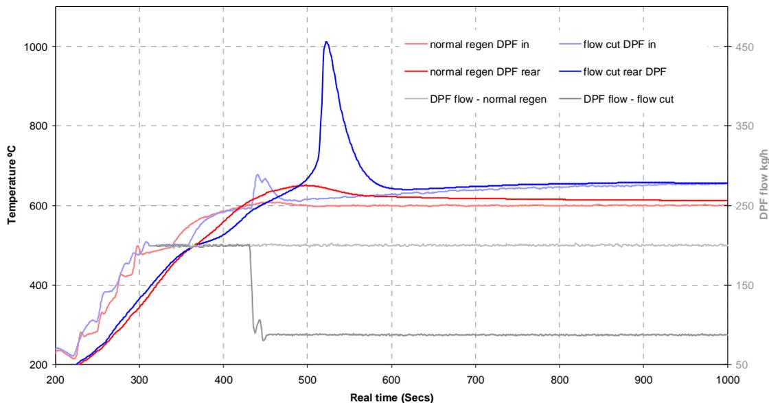
**Figure 5 Effect of flow reduction in regeneration on temperature at rear of DPF**
