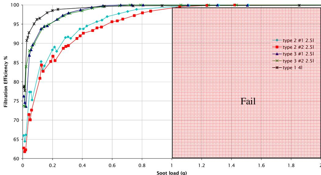
**Figure 4 Mass based filtration efficiency of various DPFs as a function of total sootload**
