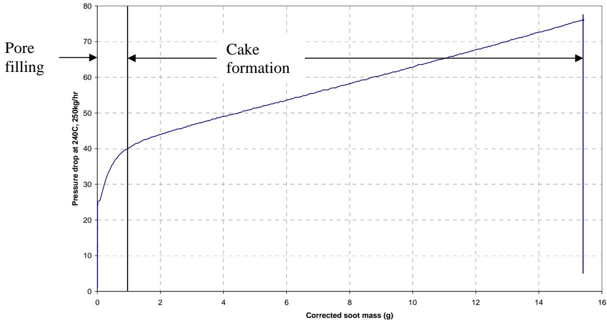
**Figure 2 Pressure Drop (mbar) vs sootload for a SiC DPF**
