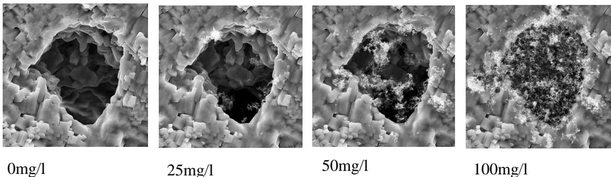
**Figure 3 30x30um SEM images of Cordierite pore of DPF loading from clean with DPG soot [2]**
