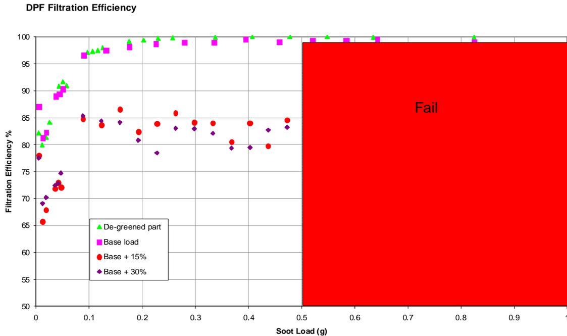
**Figure 6 Post ‘Drop to idle’ Regeneration filtration efficiency measured at increasing sootload**
