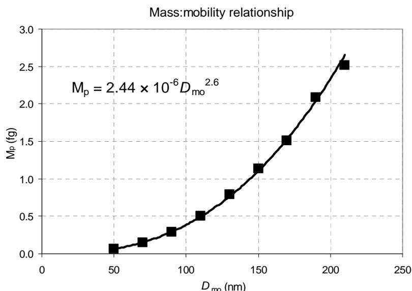
The mass:mobility relationship of an aerosol may vary with environmental factors such as humidity, as particles undergo changes in both mass and size through hygroscopic growth. The combination of CPMA and DMA allows study of these changes [Vlasenko & Mikhailov, 2013]
