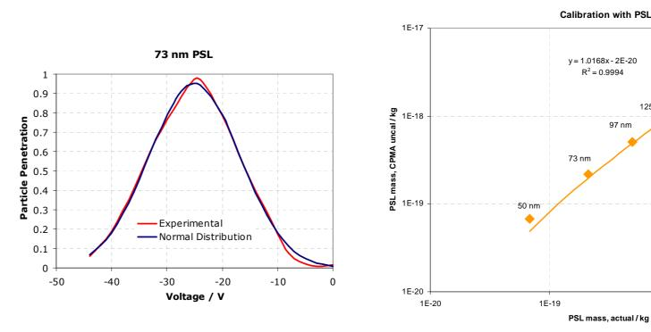
The CPMA was calibrated with traceable polystyrene latex (PSL) spheres of known diameter and density. The resultant measured masses at 50, 73, 97, 125, 152 and 220nm were compared with the known values. The source of error was deduced to be a voltage offset and this was compensated for in the engine aerosol measurements.
