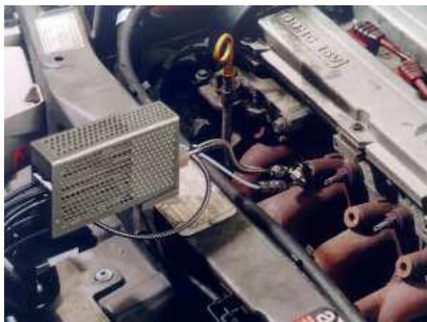
Figure 1: HFR500 sampling head and probe in exhaust port
