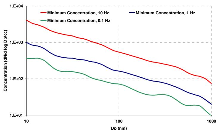
Figure 7: DMS500 Mk II Sensitivity Limits, 1 µm size range, 2009
