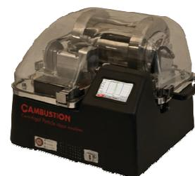
It may be considered an equivalent instrument for particle mass to the Differential Mobility Analyzer (DMA), which allows selection of particles according to their electrical mobility (drag:charge ratio).
