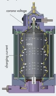
or measured by the optional Aerosol Flowmeter accessory (see below). The user can specify a constant ion concentration - time product  $(n_i t)$ , the charger will calculate and supply the optimum charging current for the given sample flow, temperature and pressure.
