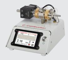
This uses the pressure drop across an orifice plate to measure the flow of particle-laden air. This enables in-situ automatic setting of the sample flow through the charger for more accurate determination of n.t.
