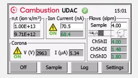
Remote control is possible via text commands to the serial or USB ports or via Ethernet. A built-in server provides VNC based replication of the touchscreen interface to a computer or mobile device.
