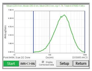
A wide range of CPCs from different manufacturers are already supported in addition to the new Cambustion 5210 CPC, which offers measurements between 5nm and 10 $\mu$ m and is ideally matched to the AAC.
