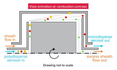
With the classifier stationary, all particles follow the sheath flow, and are lost in an internal HEPA filter.
