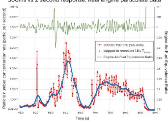
300ms vs 2 second response: Real engine particulate data
