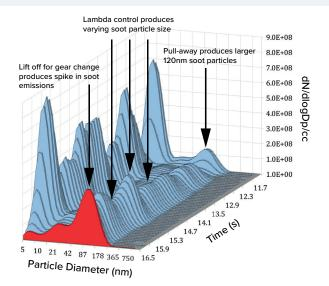
of particles falling within the counting regions for PN (>23 nm for Euro 6 and >10 nm for Euro 7). Oil consumption effects may be of particular significance for the 10-23 nm size range.
