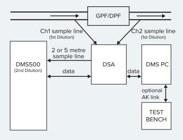
The DSA allows automated switching of the DMS500 between two different sample locations (such as pre- and post- DPF/GPF).
