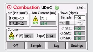
Remote control is possible via text commands to the serial port (or USB via the supplied adapter) or via Ethernet. A builtin webserver provides a Java or VNC based replication of the touchscreen interface to a computer or mobile device.
