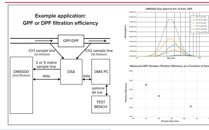
Whilst one line is selected to measure, the line which is not in use is automatically purged with clean air to avoid contamination.
