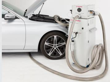
Use of the AK remote control allows programmed and unattended operation and is used for R&D and durability testing. This also allows programmed selection of the most appropriate 2nd dilution ratio in the DMS500 for measuring upstream (more concentrated soot) or downstream (less concentrated soot) of a filter.
