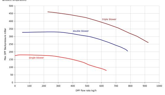
These performance specifications are for ambient temperature operation (ie in flow sweep testing) at sea level. Flow and pressure capability may be reduced by up to 30% at loading temperatures and reduced atmospheric pressure.
