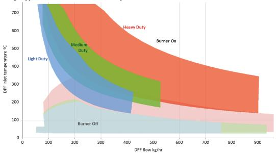
Burner off conditions are used for flow sweep testing.
