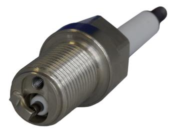
The Cambustion Sampling Spark Plug kit consists of an offset spark plug (similar to those used for incylinder pressure measurements) through which an in-cylinder heated sample probe can be fitted so that gas can be sampled from within a few millimetres of the plug electrodes. Typical applications for this equipment are shown below and include:
