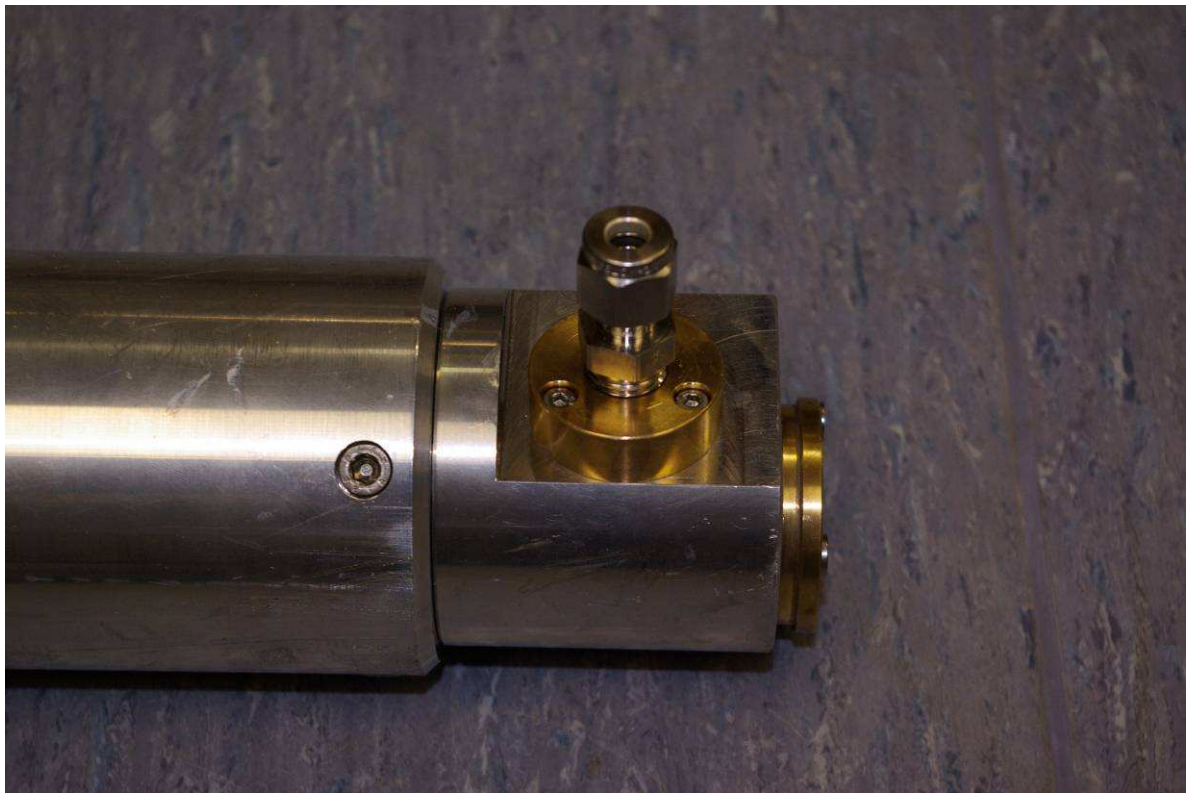
Figure 1 Heated line with SS-6M0-1-4RT Swagelok fitted
