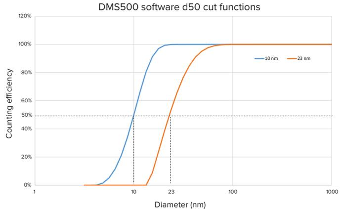
Particle losses are size dependent — measurement of the full size distribution allows automatic correction for transport losses, a correction not possible if only measuring a single concentration.
