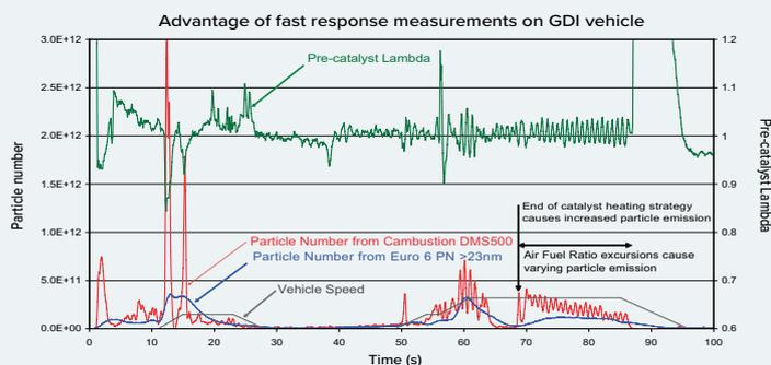
Even when fitted with a Gasoline Particulate Filter, the lower filtration efficiency achieved (due to the difficulty forming a soot cake at higher temperatures in lean conditions) on a spark ignited engine means that optimisation of engine out emissions is crucial as part of emissions compliance.
