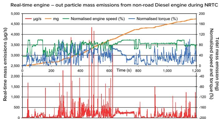
The optional Catalytic Stripper Accessory (CSA) for the DMS500 removes volatile particles from the sample. This supports enhanced accuracy as mass concentrations fall, including development for  $1\text{mg}/\text{mile}$  standards.
