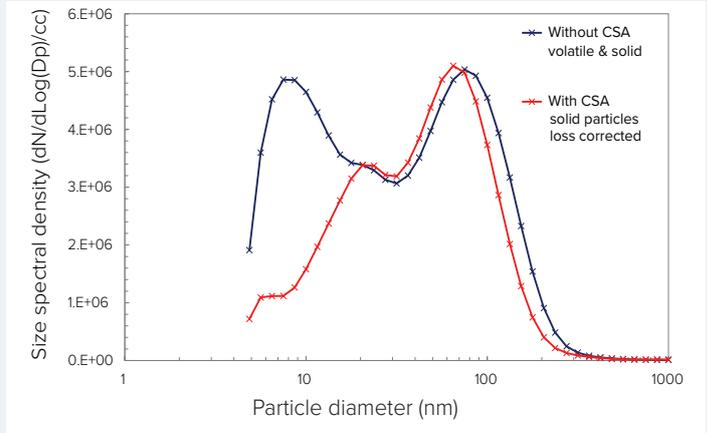
The CSA requires no additional dilution, ensuring measurement sensitivity remains unaffected. The DMS500's fast time response is also not compromised when the CSA is fitted.
