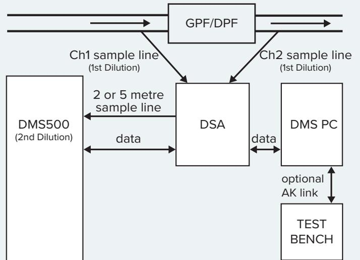
The DSA allows automated switching of the DMS500 between two different sample locations (such as pre- and post- DPF/GPF).
