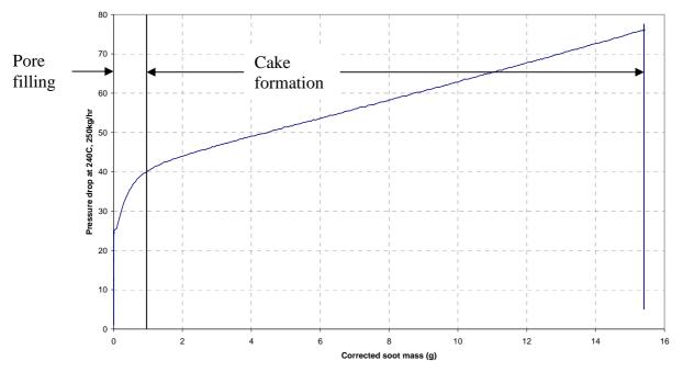
Figure 2 Pressure Drop (mbar) vs sootload for a SiC DPF
