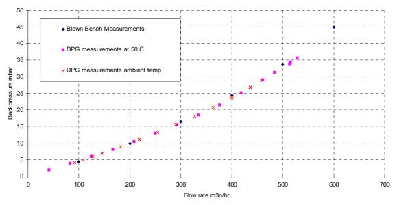
Figure 1 Pressure drop vs flow rate for DPF
