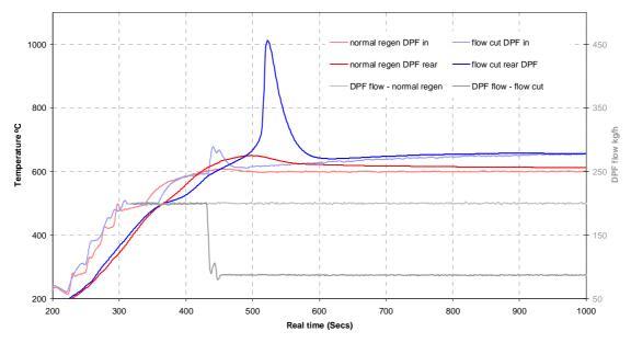
Figure 5 Effect of flow reduction in regeneration on temperature at rear of DPF
