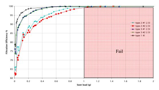
Figure 4 Mass based filtration efficiency of various DPFs as a function of total sootload
