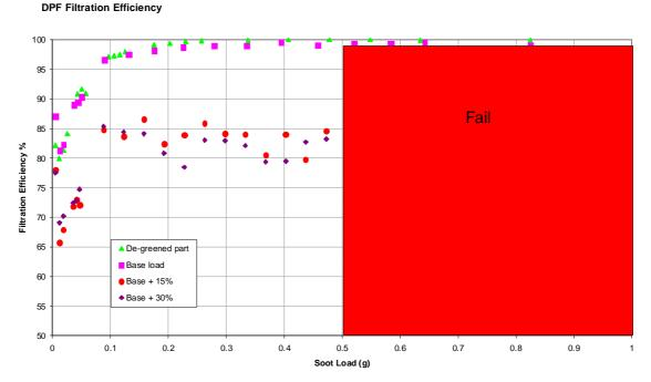
**Figure 6 Post 'Drop to idle' Regeneration filtration efficiency measured at increasing sootload** The general capabilities of the DPG for regeneration testing (including acoustic insitu crack detection) are discussed in [3].
