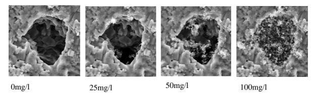
Figure 3 30x30um SEM images of Cordierite pore of DPF loading from clean with DPG soot [2]
